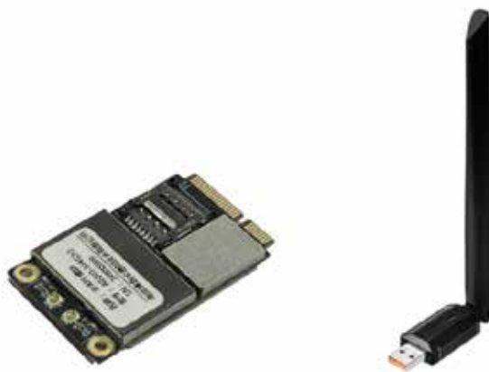
图：博洛米WAPI模块A0203-M4GX和WAPI无线网卡B0821A
